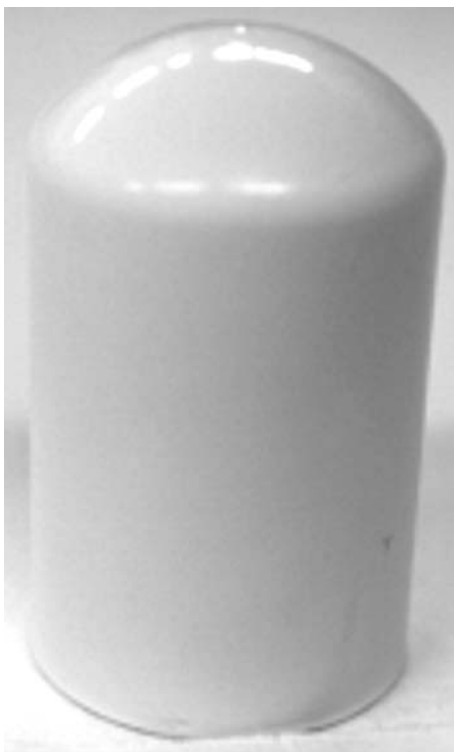
Fig. 1 Steel substrate covered by single crack-free EPD coating
