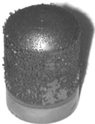
Fig. 4 Over-sintered EPD coating on a steel substrate showing the penetration of a liquid metal layer through the pores of the zirconia coating. This effect was not observed for the conditions reported in this paper
